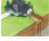
Used where adequate land space is available, horizontal loops involve one or more trenches that are dug using a backhoe or excavator. High Density Green Geothermal Pipe is inserted, and the trenches are backfilled. Each trench ranges in length up to 300'.
